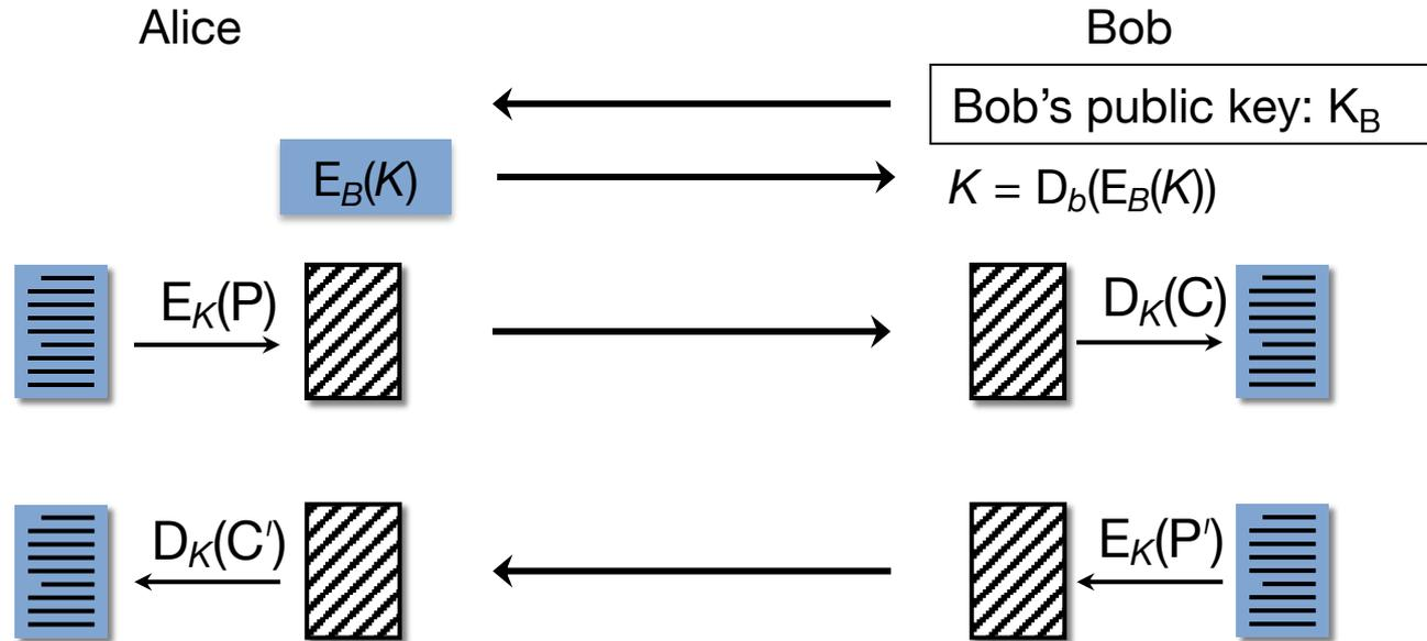
decrypt message using a symmetric algorithm and key  $K$
