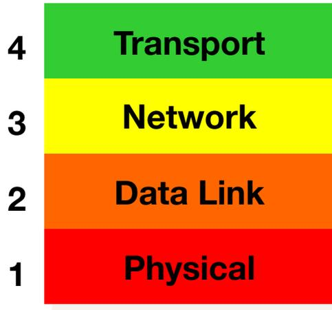
Provides an interface for end-to-end (application-to-application) communication: sends & receives **segments** of data. Manages flow control. May include end-to-end reliability
